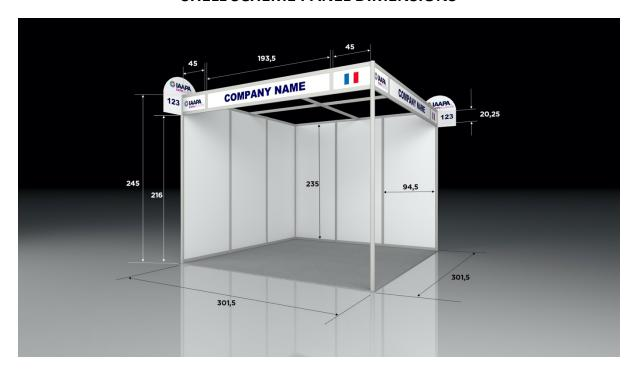
The illustration shows a 3m x 3m stand open on two sides.
