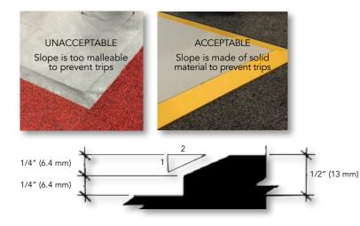
Changes in level greater than 1/2" (13 mm) are required to be ramped. To accommodate the widest range of users, ramps should have the least possible running slope, which may not be steeper than 1:12.
