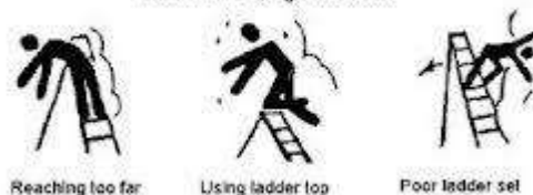
Ladder Riding Hazards
